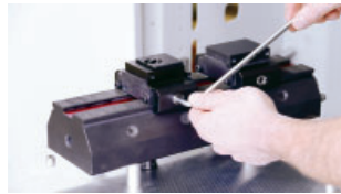
Example of pull-down elements (Diagram G)
