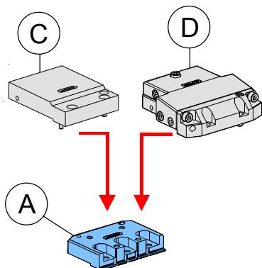
Determine the position of the workpieces on EROWA PreSet 3D or EROWA PreSet Basic Uno PalletSet W and transmit data to the WEDM center.
